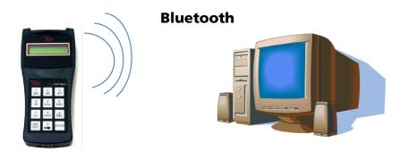
When connecting the Brake Meter for the first time using the Bluetooth interface, user will need to configure the Bluetooth connection. To configure the Bluetooth connection, open your Bluetooth manager program on your PC and search for Mini+##### device, where '######' is the serial number of the brake meter.
