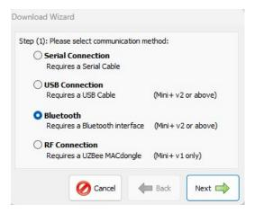
Select the COM port number of the Bluetooth connection connected with the brake meter. The COM port number is the same COM port obtained during the Bluetooth pairing process.
