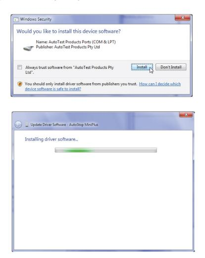
When Windows has completed installing the drivers for the USB interface, the following window will appear. Notice the COM port number displayed on the titlebar. The COM port will be used when downloading data from the meter using the datalogger software.
