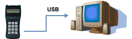
Once the USB cable is connected to the PC, switch ON the Brake Meter by pressing the ON/OFF key. When the Brake Meter is switched ON, the PC will recognise the Brake Meter device and will search for the USB drivers.
